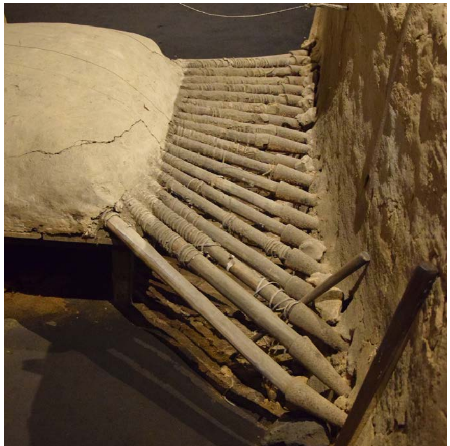
Model of a tataru furnace, tuyeres
