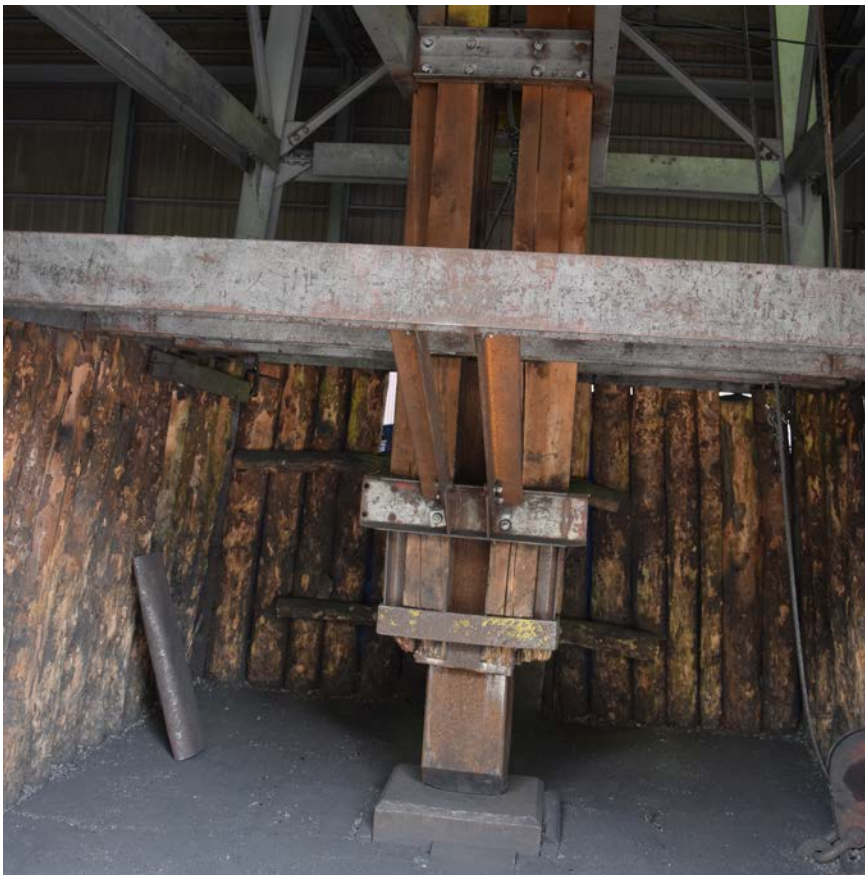
Hammer used to crush the kera block, Nittoho Tatara Factory
