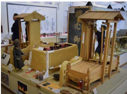
Model of a tataru furnace with bellows on each side, Itohara Memorial Museum
