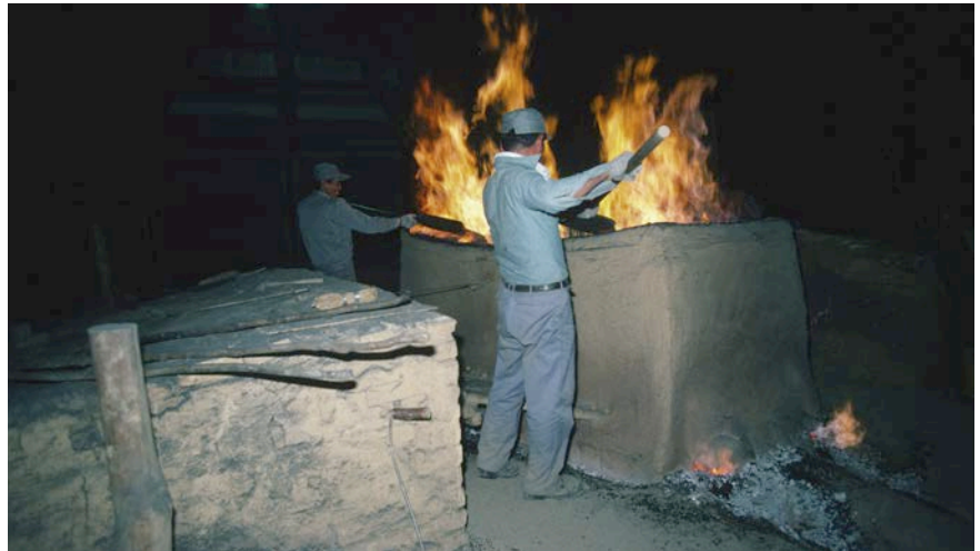
Pouring iron sand and charcoal into the furnace
