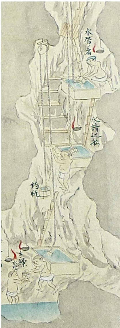
Draining the mine with buckets and hoist, Sado kozan kyushiki kogyo zu Courtesy of Kyoto University, Faculty of Engineering, Library Sign. 56114
