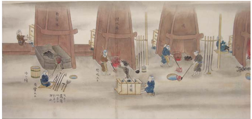
Three kinds of furnaces for different stages in the smelting process. The one on the left is said to go back to western origins; behind each furnace is a wooden bellows operated by hand, Courtesy of TU Freiberg
