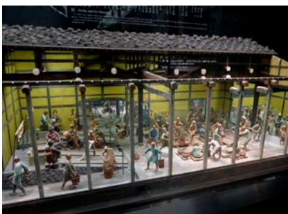
The yose seriba workshop for concentrating and smelting gold ore; this model in the Sado Gold Mine Museum shows the crushing, grinding, and washing of gold ore, which later was smelted and refined ©R. Mathias
