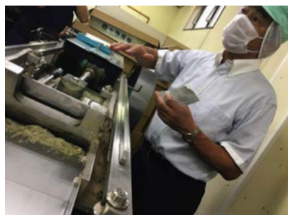
Aimono demonstrates his slicer that cuts to a fraction of a millimetre
