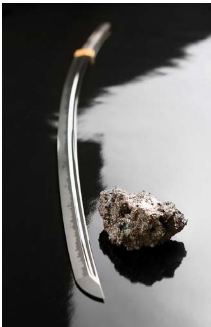
Less than half the total number of pigs of steel (tamahagane) are suitable for making the finest Japanese swords
